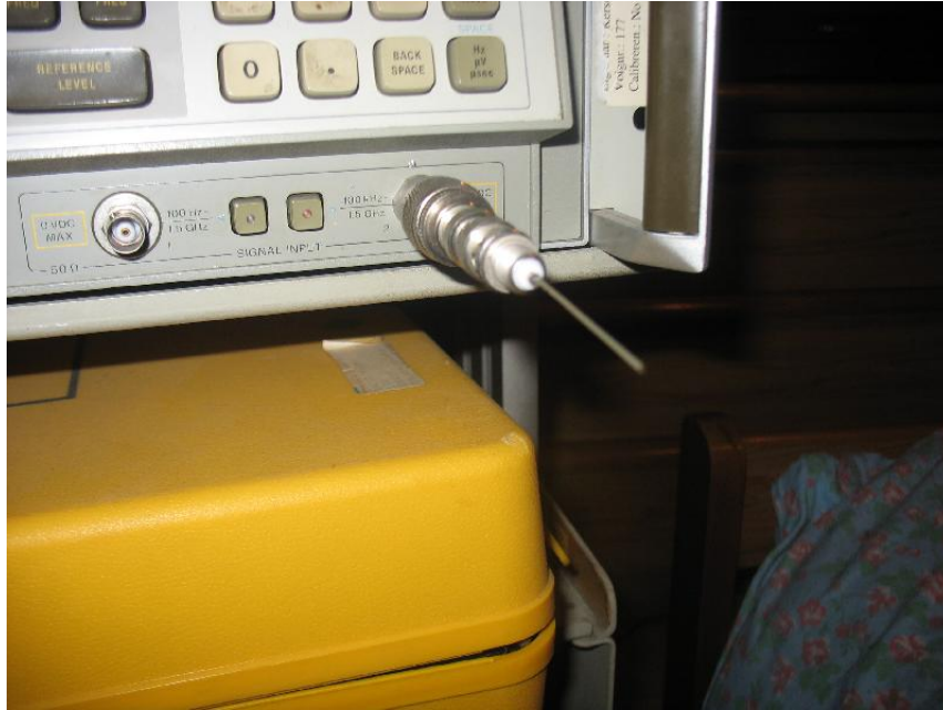
Magnetic antenna probe to measure the magnetic field
